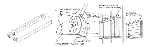
Fan and tube ventilation give positive air flow while polyethylene ducts distribute the incoming air evenly throughout the greenhouse. The plastic ducts are suspended by wires or straps from the roof of the greenhouse.
